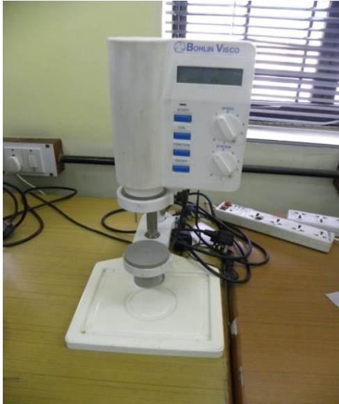
Viscometer (Cone and plate type)
