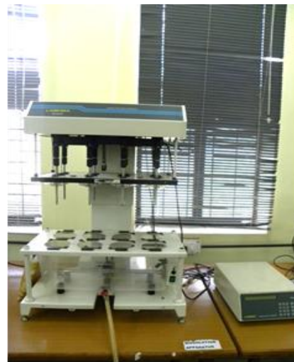
Eight Station Dissolution Test Apparatus (USP Type I and II)
