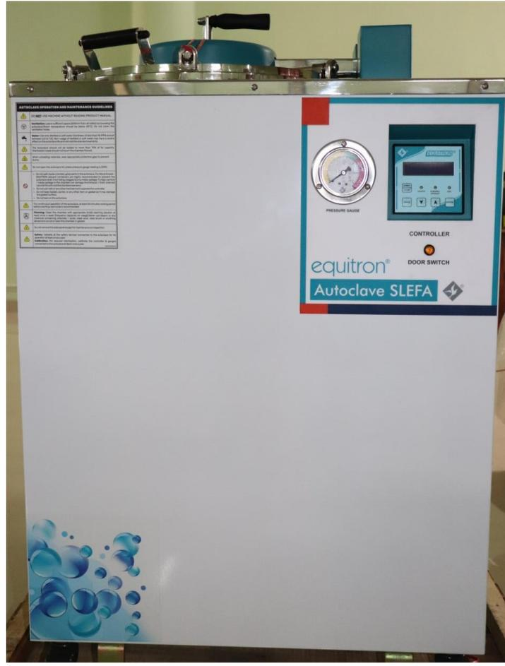
Autoclaves provide a physical method for disinfection and sterilization with a combination of high temperature, steam, pressure and time in order to kill infectious microorganisms and spores. They are also used to decontaminate certain biological waste and sterilize media, instruments, lab ware, medical waste that might contain bacteria, viruses and other biological materials that are recommended to be inactivated by autoclaving before disposal.
