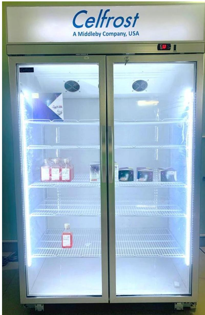
These refrigerators are used for maintain a cold storage conditions for samples, chemicals specified to be stored at 1-8 °C.
