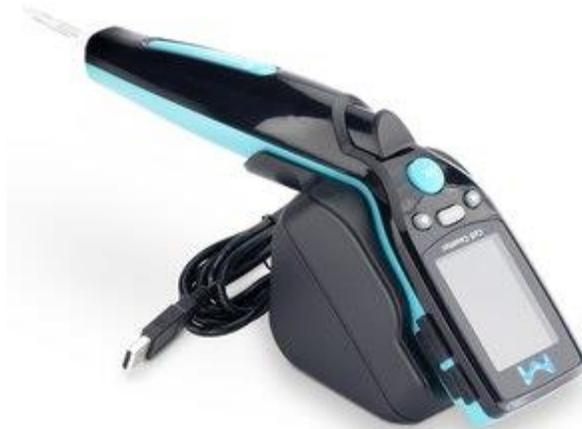
The Scepter Cell Counter is used to perform a fast and convenient cell counts in an easy to use format. This instrument is used in sampling process where it reveals data on cell concentration, average diameter, average volume and histogram displaying population information on your culture within 30-40 seconds. The time to perform the cell counting experiment has been reduced from approx. 10-15 minutes in conventional cell counting systems to less than 30 seconds by the
