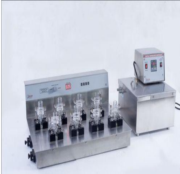
Eight station jacketed Franz Diffusion cell apparatus
